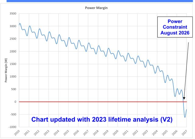
Gradual decrease in Power Margin as the Solar Array (SA) power generation capacity decays due to known and anticipated SA degradation. Several factors play role in SA power generation degradation due to long-term exposure to low Earth orbit. The Power Margin is zero when the power generation capability of the SA just meets the spacecraft and instrument operational load. This is predicted to occur in August 2026 according to the modeling of future string losses.
