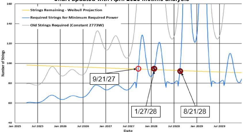
Projected number of solar array (SA) strings (yellow line), estimated number of strings required to generate a fixed power of 2,773 Watts (W; gray curve), and estimated number of strings needed to operate all instruments based on the average power generated per solar string according the EPS ARE SOH test results (blue curve), for the period 2025-2030. FOT analysis indicates that the SA will be capable of generating the minimum required power for spacecraft bus operations until 9/21/2027.
