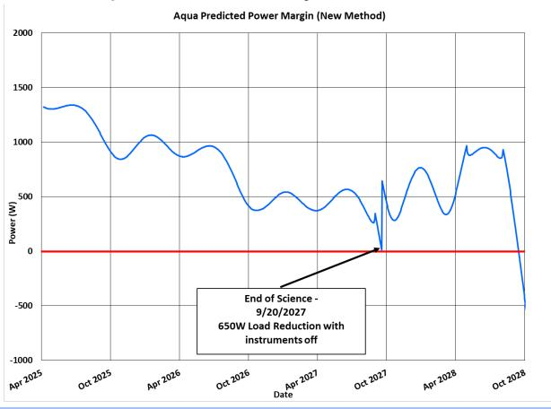
Gradual decrease in Power Margin due to the combined effect of orbital drift and reduction of Solar Array (SA) power generation capacity as the SA degrades. Several factors play role in SA power generation degradation due to long-term exposure to low Earth orbit. The Power Margin is zero (red line) when the power generation capability of the SA just meets the spacecraft and instrument operational load.
