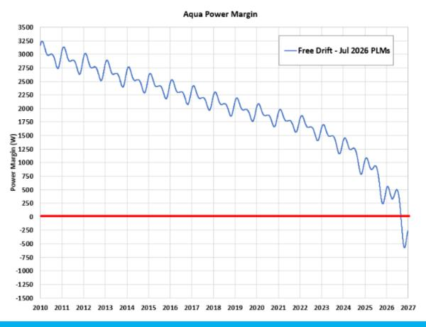
Gradual decrease in Power Margin as the Solar Array (SA) power generation capacity decays due to known and anticipated SA degradation. Several factors play role in SA power generation degradation due to long-term exposure to low Earth orbit. The Power Margin is zero when the power generation capability of the SA just meets the spacecraft and instrument operational load. This is predicted to occur in September 2026 according to the modeling of future string losses.
